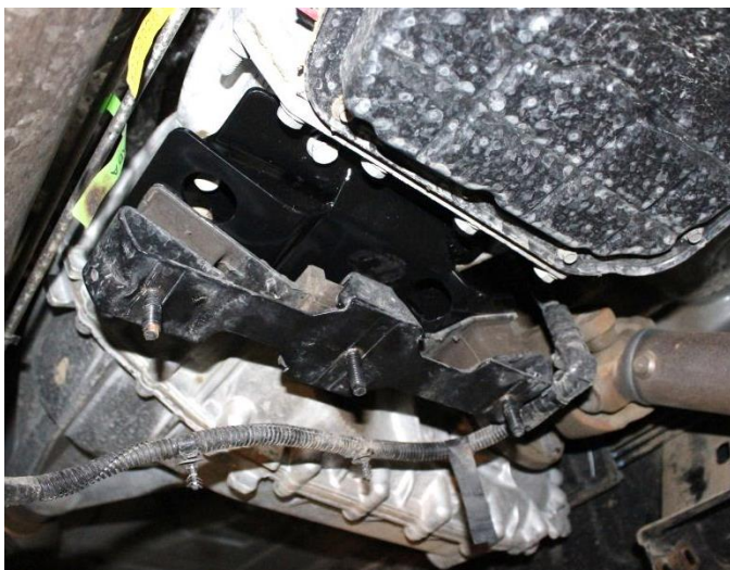
16) Reinstall the transmission mount into the truck using the factory hardware.
