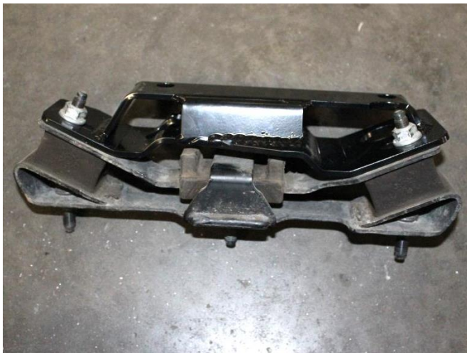
16) Reinstall the transmission mount into the truck using the factory hardware.
