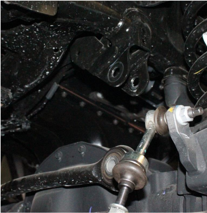
14) Remove the front upper nut and the lower bolts securing the shock to the axle. Save the lower Hardware. Remove shocks.
