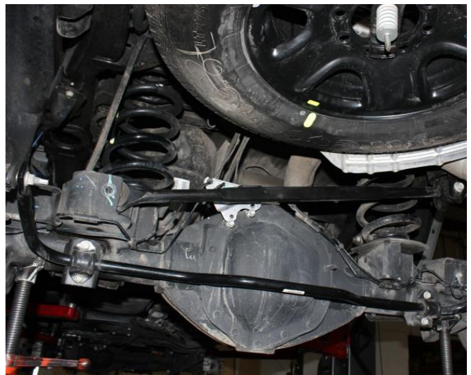
9) Enlarge the holes in the lower coil mounting plate to 7/16"
