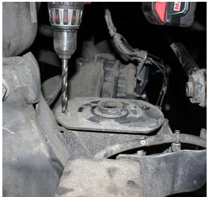
9) Enlarge the holes in the lower coil mounting plate to 7/16"
