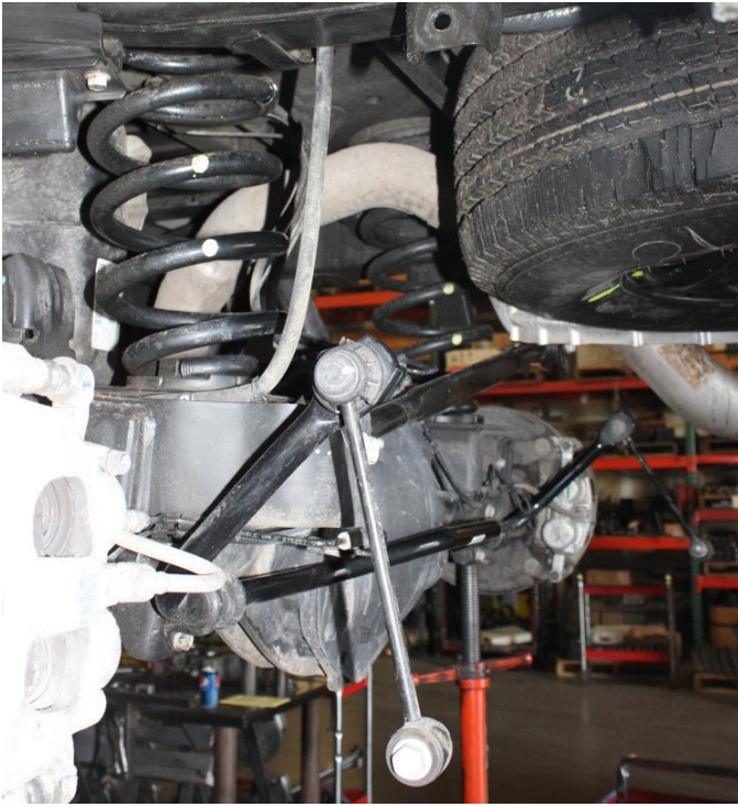
6) Disconnect the rear track bar from the axle, retain all hardware.
