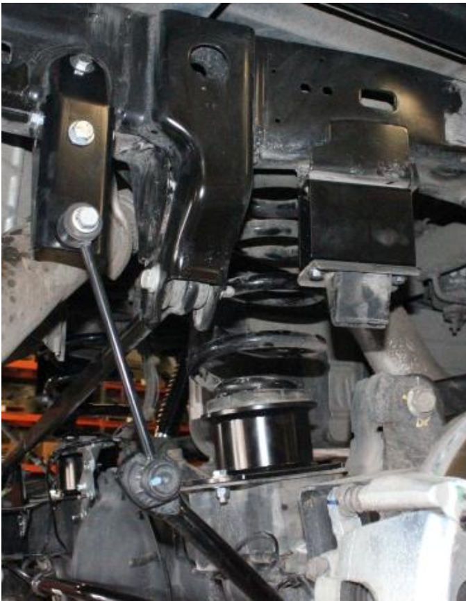
24) Install rear brake line bracket as shown.
