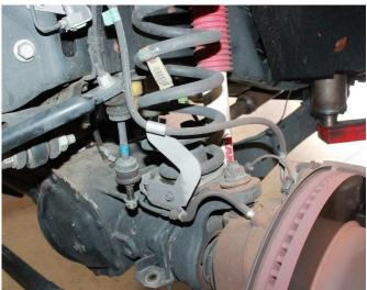
4) Remove hardware attaching ABS wire to the lower coil mount. As shown below.
