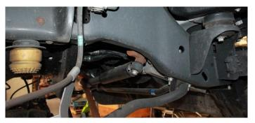
8) Disconnect the trac bar from the frame bracket.
