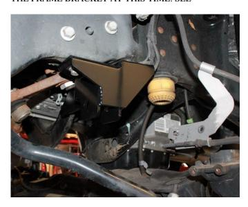
11) Remove the bolt attaching the Radius arms to the factory frame mounts. Save the factory hardware.
