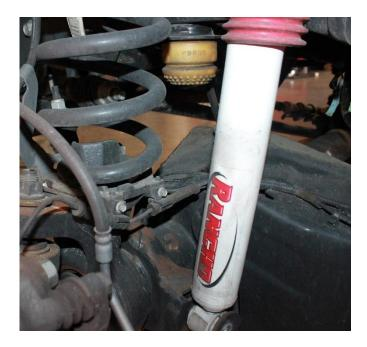
5) Remove the front shocks and save for Reinstallation, save hardware.
