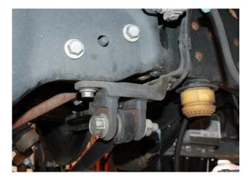
9) Remove the trac bar bracket from the frame, save the original hardware and discard the factory trac bar bracket.
