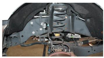
7) Disconnect the factory steering stabilizer from the frame mount.
