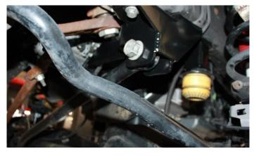
25) Reconnect sway bar to the front axle using factory hardware as shown below.
