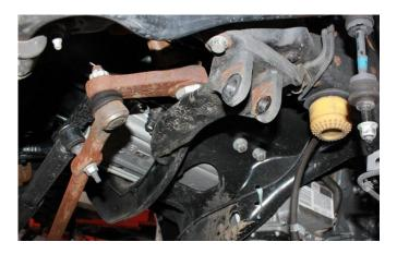
10) Track Bar Bracket). Attach to the frame using the original hardware in the same position. Torque bolts to 120 ft.-lbs. DO NOT ATTACH THE TRAC BAR TO THE FRAME BRACKET AT THIS TIME. SEE
