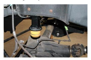
17) Remove the factory lower coil mount, save hardware for Reinstallation.
