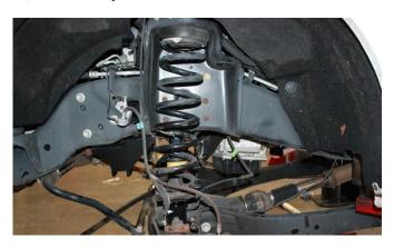
22) Install the front shocks extenders using the supplied factory hardware.
