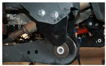
13) Reinstall the radius arms into the new drop down bracket using the factory hardware. Attach to the axle first then to the new drop bracket using the upper most hole. Torque to 250 ft.-lbs.
