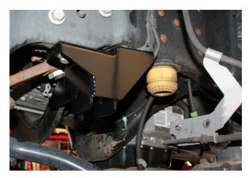
15) Drill out the factory bump stop cup to 3/8" as shown below.
