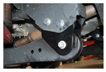
14) Working from both sides of the truck, Remove the factory front bump stops and save. Pull on the bump stop itself to free from the cup. Remove the factory mounting cup from the frame and discard the hardware.
