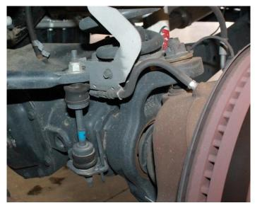
3) Disconnect the brake line from the frame and axle on both driver and passenger sides. Save hardware.
