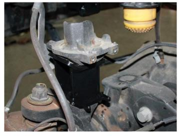
19) Remount the ABS wires using the factory hardware as shown below.
