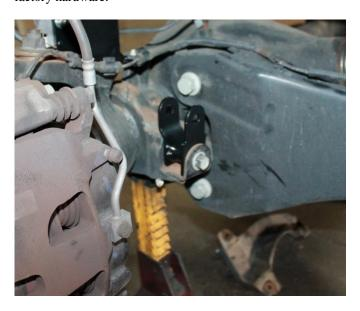
23) Install the front shocks using the supplied  $9/16 \times 3$   $\frac{1}{2}$  hardware.
