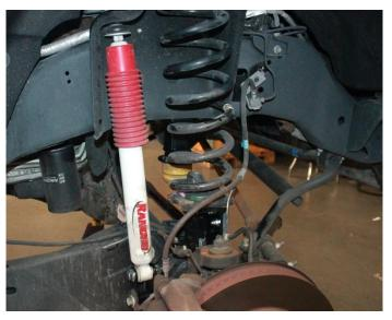
24) Position the factory trac bar into the new trac bar bracket. Note: You may need to raise the axle up or down to align the hole. Using the original bolt, insert it from the front side of the bracket towards the back. Torque the trac bar bolt to 400 ft-lbs.
