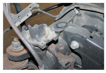
18) Install lower spacer as shown using the 14mm x 25mm hardware, Use Loctite. Install coil mount to spacer using factory hardware and supplied 14mm nylock nut.
