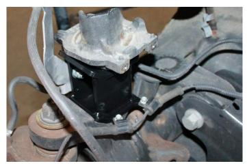
20) Mount the brake line bracket to the front side of the lower coil spacer using the supplied  $5/16 \times 1$ " hardware as shown below.
