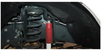
6) Lower the front axle allowing the coil springs to come free of tension and remove the coil springs. EXERCISE EXTREME CAUTION WHEN WORKING WITH COIL SPRINGS UNDER LOAD!
