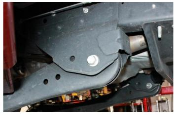
12) Install the radius arm drop brackets. Place the brackets into the factory radius arm pockets. Attach the bracket to the factory bracket using the supplied  $\frac{3}{4}$ " x 1- $\frac{3}{4}$ " bolts, nuts and washers through the original holes in the frame. Torque bolts to 240 ft.-lbs.
