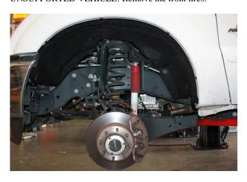
2) Disconnect the sway bar from the sway bar end links. Save hardware. As shown below
