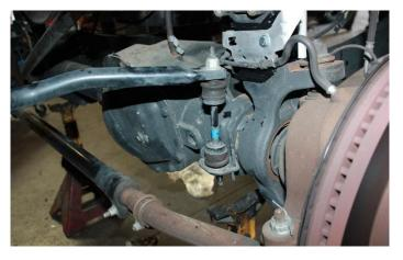
26) Remove hardware connecting sway bar u clamps to the frame and install sway bar drops as shown below using the  $7/16 \times 1^{1/4}$ " hardware.
