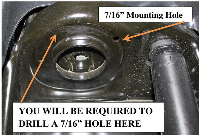
2) Using the supplied 7/16" x 1 1/4" bolt and washer, Install the bolt thru the coil spacer then thru the frame
