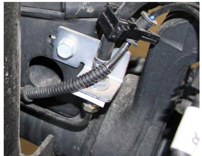
8) Reconnect factory swat bar using factory hardware.
