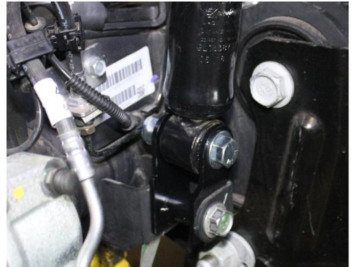
5) Raise the floor jack until the spring is in the proper compressed. Install the shock into the shock extension using the 9/16 x 3 1/2" bolts and hardware. Torque to 95 ft.-lbs.
