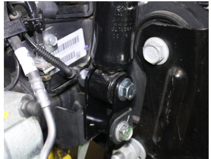
6) Reinstall the brake line bracket to the lower coil perch using factory hardware. Torque to 20 ft.-lbs.
