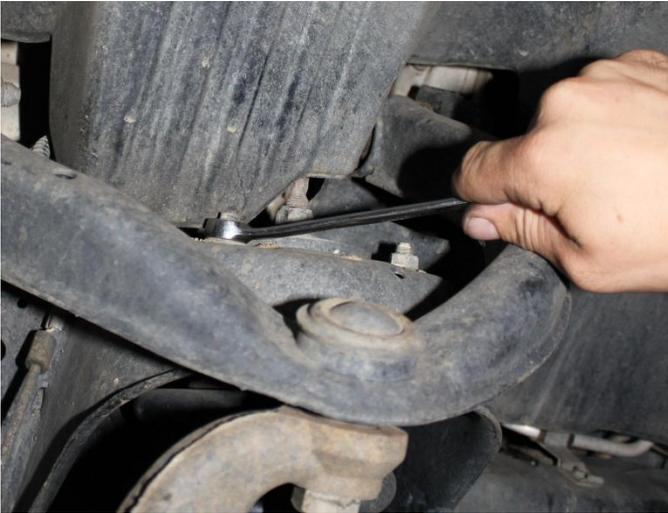
7) Loosen upper ball joint nut.
