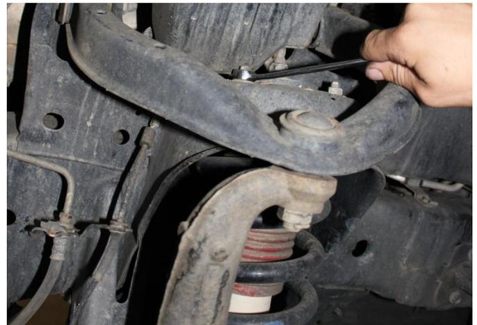
12) Push suspension down and remove strut from vehicle.
