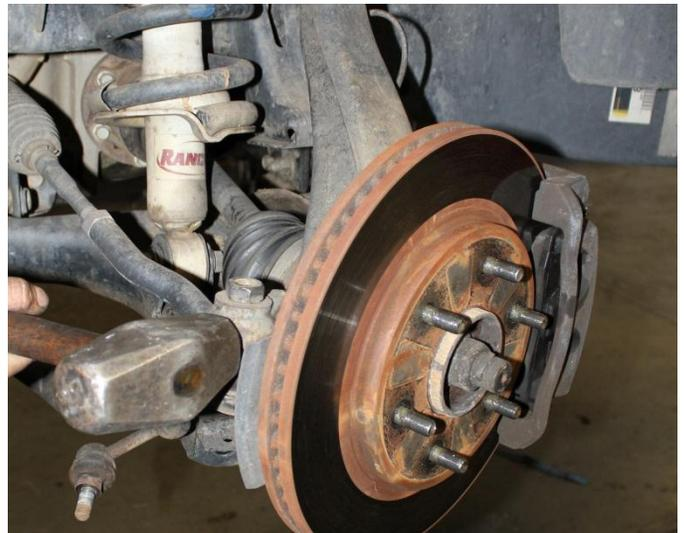
10) Strike the steering knuckle to dislodge the upper ball joint. Remove ball joint from knuckle.
