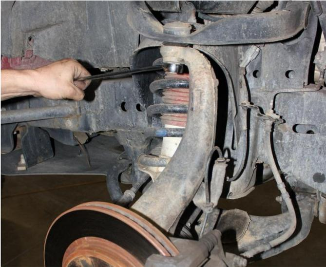
18) Reconnect outer tie rod. Insert new cotter pin.
