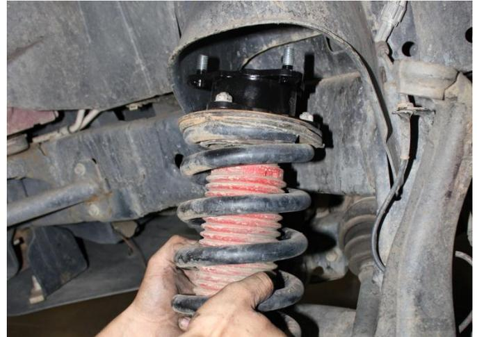
11) Remove lower strut mounting bolt/nut
