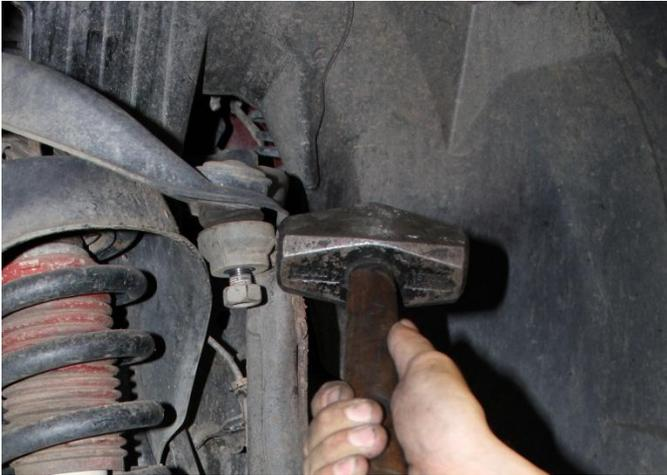
14) Strut assembly will be rotated 180 degrees for re-installation.
