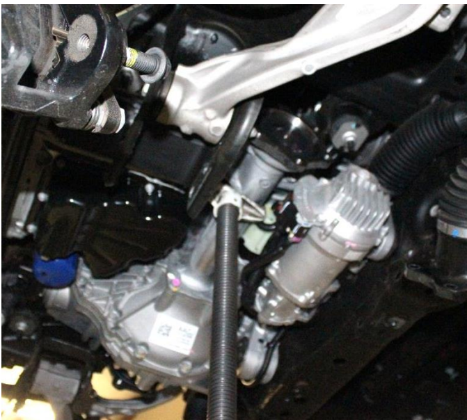
18) Remove the mounting hardware at the four mounting points of the differential.
