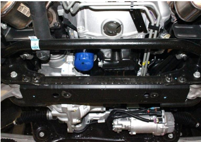
17) Support the front differential and remove rear cross member.
