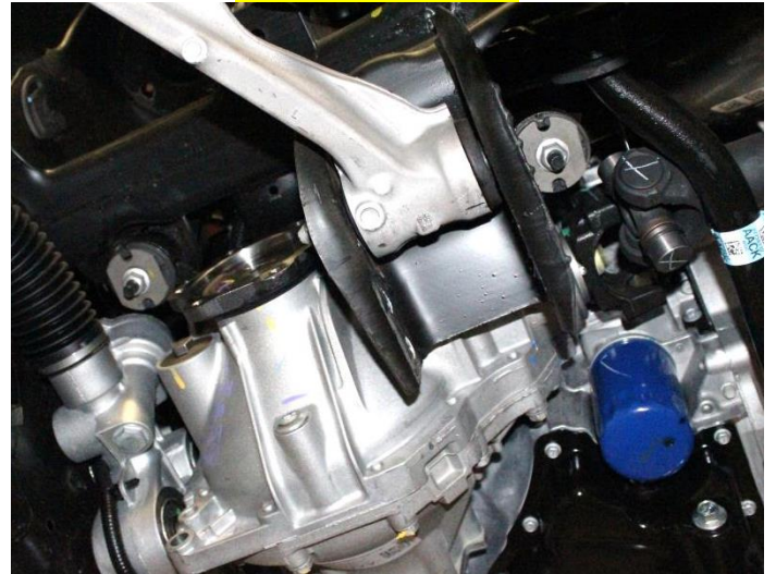
19) Use the .950 spacer in the front and the .750 on the rear mount.
