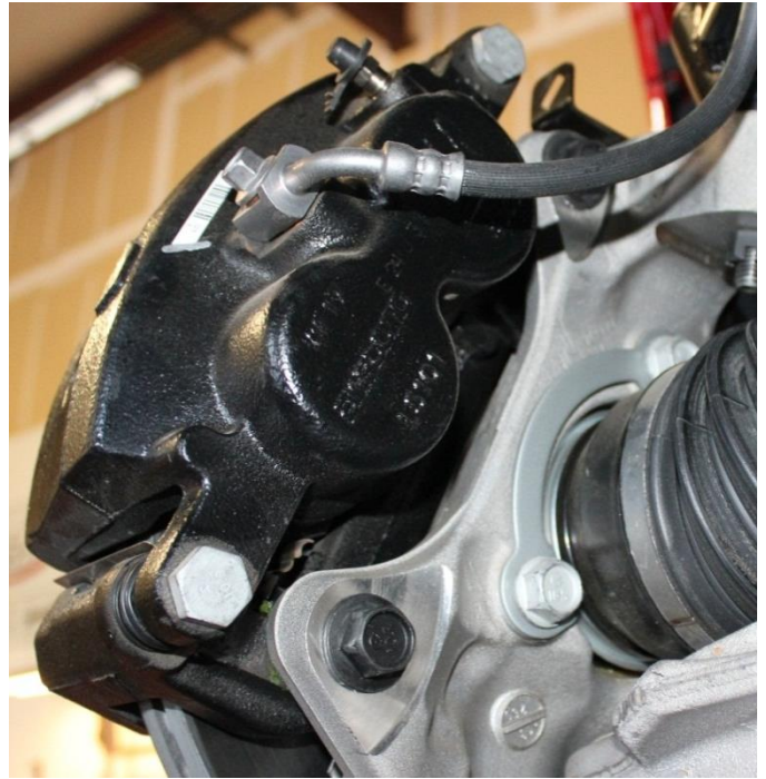
35) Reconnect the inner CV shaft using the factory hardware. Tighten to 45 ft-lb.
