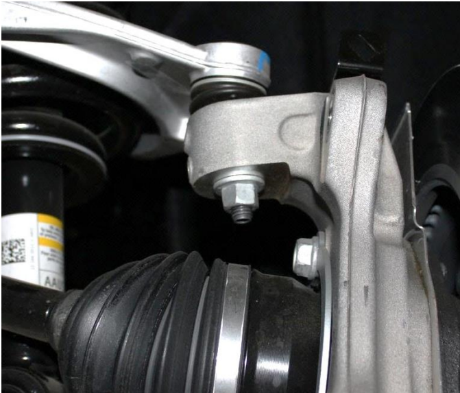
10) Remove the six 15mm axle shaft bolts. Set the hardware aside as it will be reused. Repeat on opposite side
