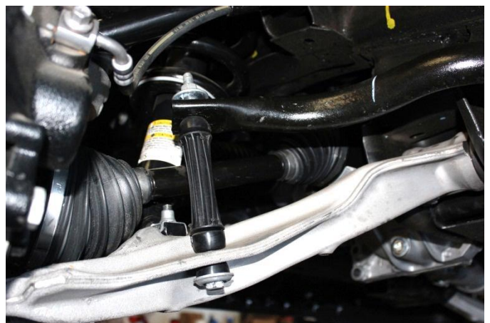
37) Install the brake line support bracket onto upper control arm using the 1/4" nuts and washers provided. Tighten to 7 lb.-ft.
