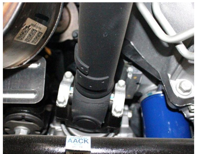
15) Disconnect the front drive shaft from the differential, Don't Remove the drive shaft. Slide the driveshaft back off the yoke.
