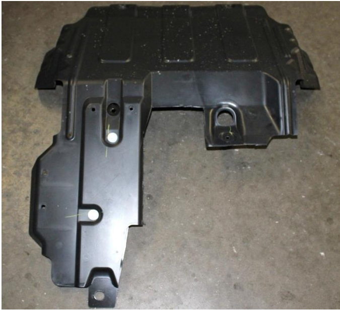
41) reinstall factory skid plate as shown. Install the 5/16" x 1" hardware as shown below.
