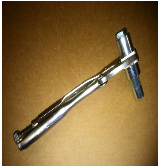
THIS IS THAT THE TOOL WILL LOOK LIKE TO INSTALL THE INSERT
