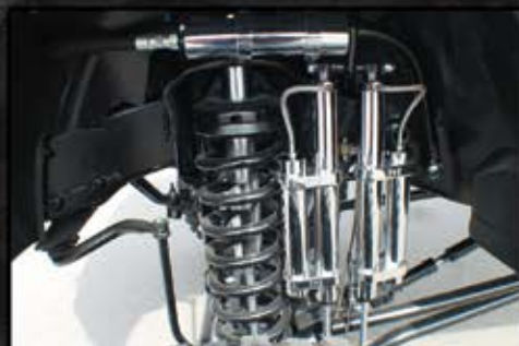
2.5 Coilover with Large Diameter Ring Designed to run a factory diameter Coil
